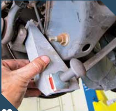
**09** The forward horizontal shock bracket in the Stage II kit simply bolts in using existing hardware in the rear suspension's sway bar and track bar. The shock can then be installed to complete the job.
