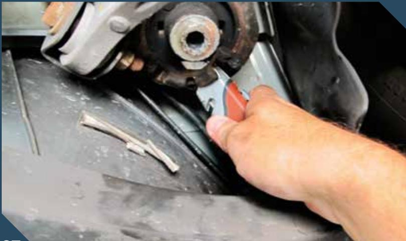
**05** Trimming the factory rubber bushing for the proper fit is the most time consuming part of this installation, but we accomplished it in fairly short time using a razor knife. Changing blades frequently helps as the rubber really seems to dull the blade.
