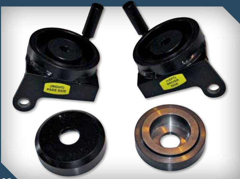
**02** Hop Not fabricates CNC steel spacers that eliminate the movement allowed by the factory rubber bushings. This is a simple idea, but very effective and doesn't require dropping the rear cradle or re-aligning the rear suspension. The Stage I kit includes spacers for all four cradle attaching points.
