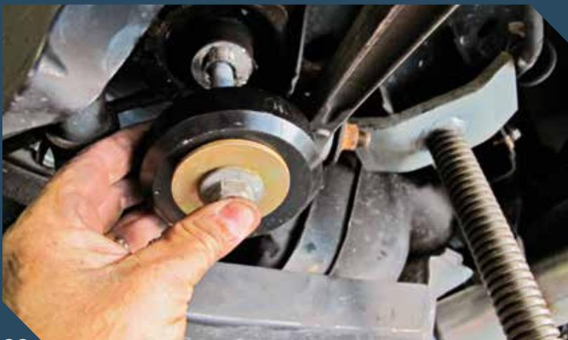
**06** Once the rubber is trimmed away, the Hop Not spacer can be installed using the factory bolt. This spacer forms a solid mount between the factory inner bushing sleeve and the outer diameter of the rear cradle, eliminating movement allowed by the factory bushing.
