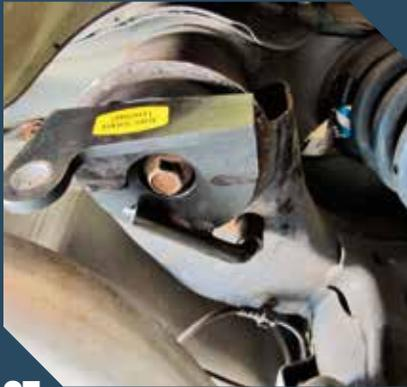
**07** The rear Hop Not spacers use an existing hole in the frame rail for proper location. Our Stage II kit rear spacers have provisions for the rear horizontal shocks. Again, you'll have to trim a little of the stock rubber bushing for proper fit.
