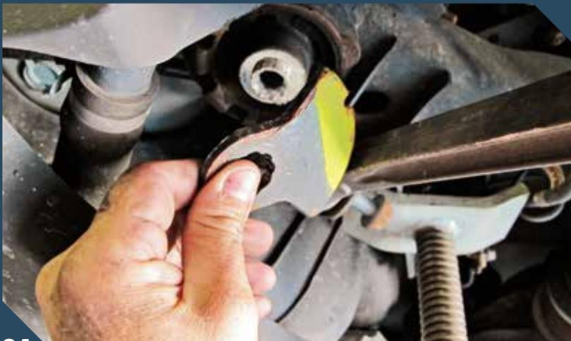
**04** The spacers are installed one at a time, and by using the factory bolt and provided spacer tool the front triangular steel plates can be pried off the rubber bushing. The OEM rubber bushing is then trimmed so the Hop Not spacer fits properly.
