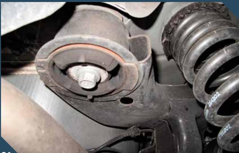
**01** The rear cradle holding the independent suspension to the car is held in place by large, soft rubber bushings. While these bushings likely improve ride quality and dampen harmonics, they allow the entire rear cradle to move, which is counterproductive in terms of straight line or cornering performance.
